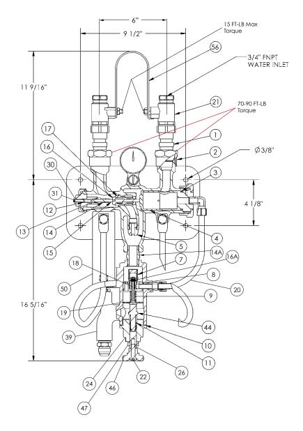
desired temperature. Turning the knob (46) clockwise lowers the temperature and turning it counterclockwise raises the temperature.
