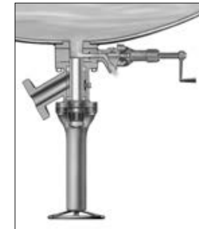
Fig. 2 - Drain Valve Open for Sample
